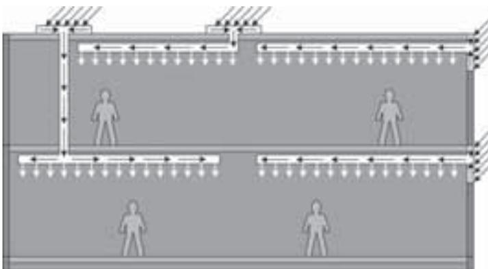
Figure 1. Sunlight is collected on the rooftop or façade and piped inside for lighting.
