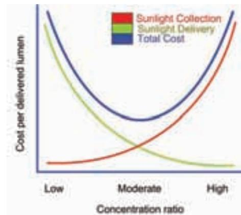
Figure 2. Optimal system cost depends on choice of sunlight collection and delivery approaches.
